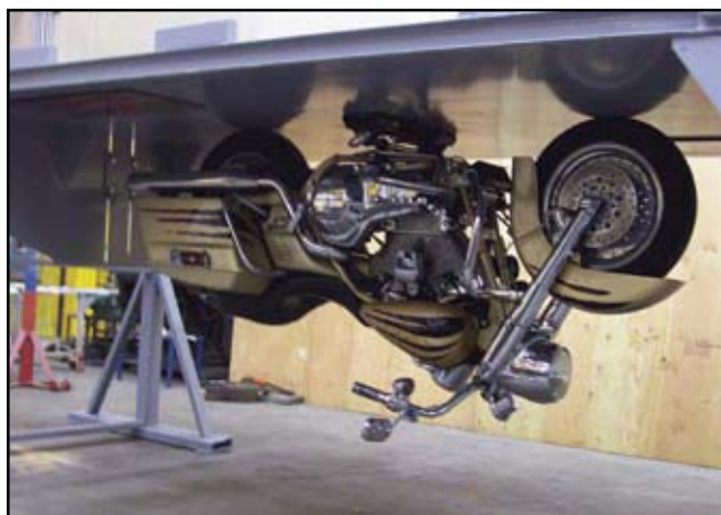
This "motorcycle rotisserie" was constructed to test the Frame Lock® system and demonstrate the unequalled security it offers. Would conventional straps hold this hog on the trailer? (Visit www.sscycle.com to see a video of this "rotisserie" in action.)
