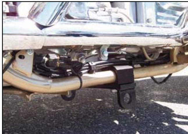
The pin bracket can be installed on the frame clamps in minutes. It is just as easy to remove before the bike is ridden.
