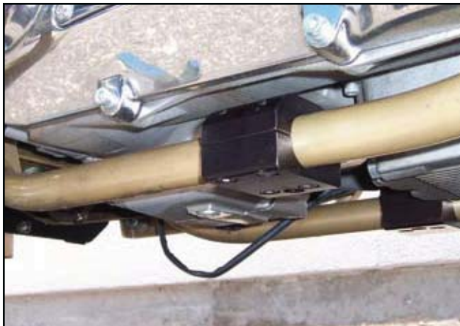
Clamps installed on the frame.
